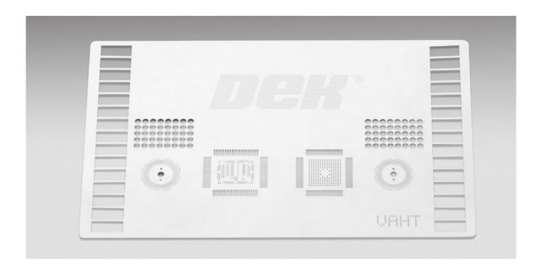
Electroform stencils can be produced with modifications to accommodate specific applications. One such adaptation is a technique called Variable Aperture Height Technology (VAHT), whereby a gasket overgrowth is created around apertures to create more aperture height to allow for increased paste volumes to be deposited.
