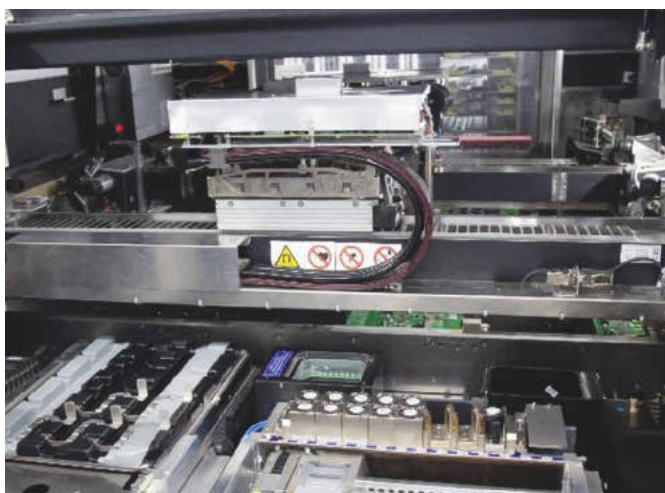
The Siplace SX as it takes busbars from trays
