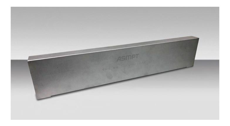
DEK support bars serve as a quick and universal support solution for PCBs to be printed on one side only and other substrates. The operator places the DEK support bar manually on the printing table between the conveyors. That way, a wide range of PCBs and substrates can be printed after a short setup time.
