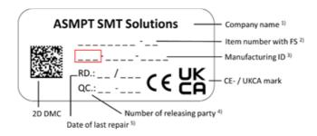
re. 3): The connector designation from the item's product-specific documents must be specified in the block marked in red. The connector designation is omitted for cable ends without a mounted connector.
