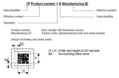
The blank zone (BZ) must be implemented as a function of the barcode resolution (X) as  $\geq 2X$ .
