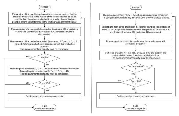
If the required machine or process capability is not achieved, a 100% inspection must be performed for the attribute in question.
