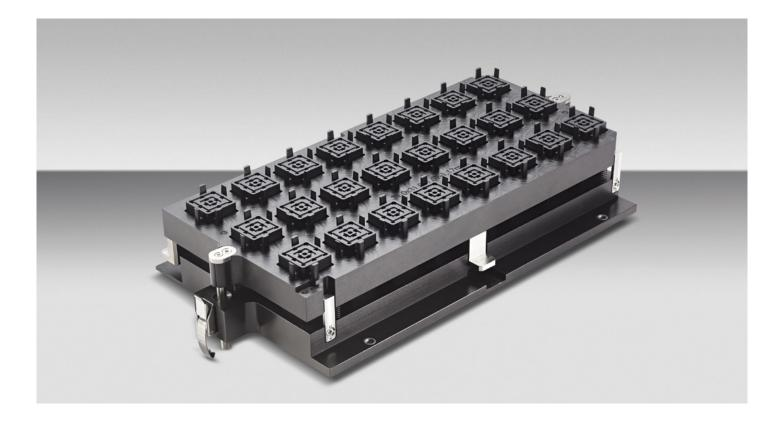
DEK Virtual Panel Tooling (VPT) allows the printer to process multiple individual substrates in a single print cycle. The substrates are presented to the printer in a carrier and are then lifted out, mechanically centered (aligned) and placed into a surrounding plate to create a "virtual panel" prior to coming in contact with the stencil and then mass imaged.
